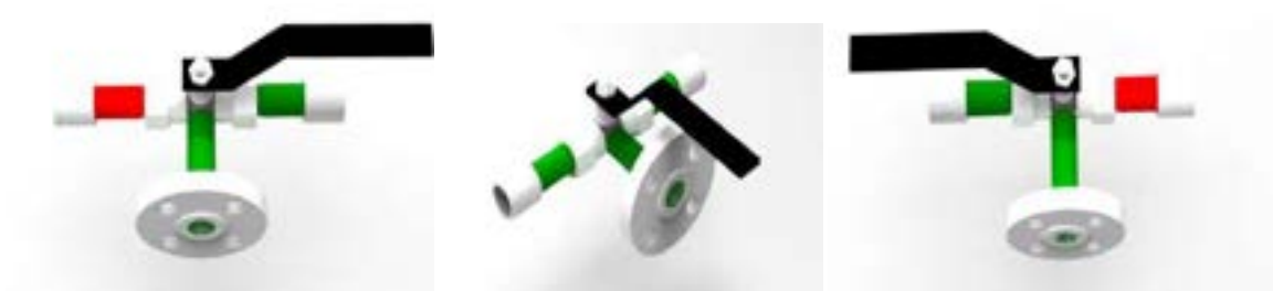
Image H: 3 Positions of a T Port Ball Valve.
